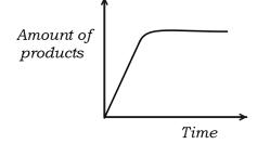
At the beginning, the amount of the product is low and increases as time goes on. As the reactants get used up, the reaction slows down and when there are no more reactants the reaction stops and the curve becomes horizontal/constant. At the point where the curve becomes horizontal, it means that the maximum amount of the product has been formed.
