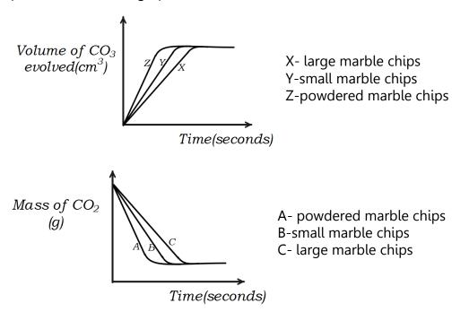
Instead of plotting volume of gas evolved against time, the mass of the solid can be plotted against time as shown above.
