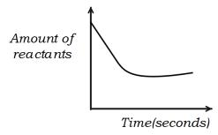
From the above graphs, the rate of reaction at any time is determined by calculating the gradient of the tangent of the curve at that time
