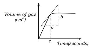
From the graph, the rate of reaction at time  $t = \frac{\text{change in volume}}{\text{change in time}} = \frac{b}{a}$
