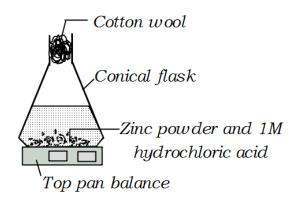
The experiment can be repeated using the same mass of zinc and the same volume of HCl with different concentration. A graph of mass of flask and its contents against time is shown below
